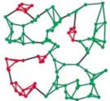
Computation of a minimum cut that separates a network into two components (i.e., the most fragile part of the network). A cut with size two can be found around each red cluster.
