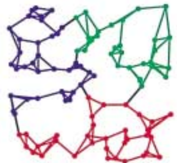
Computation of a minimum cut that separates a network into three components with the same number of vertices.
