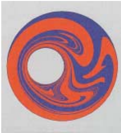
An efficient mixing of fluids is attained if two eccentric cylinders are rotated alternately so that each fluid particle moves chaotically. This is called a chaos mixing.
