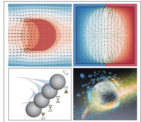
Unidirectional flow around a heated U-shaped body (top left)
