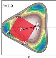
Rotary ratchet model consisting of a rotor (rigid body consisting of four points) and a rotor housing (potential) that simulates a Wankel rotary engine
