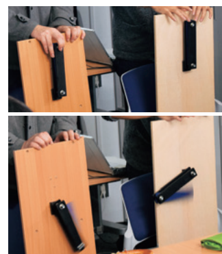
Double pendula showing chaotic motion:
