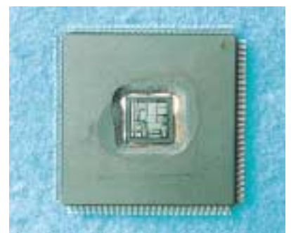
An MPEG2 decoder LSI synthesized by PARTHENON system.
